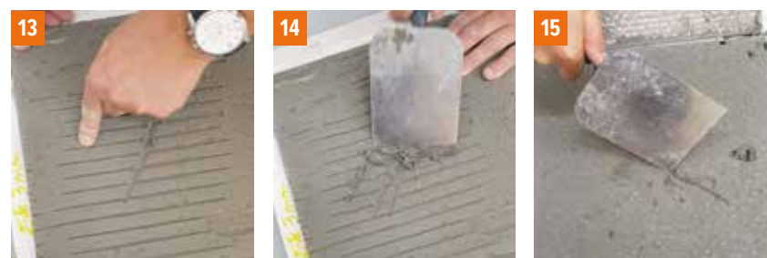
Photos 13, 14, 15 Geoflex Express. The first two photos show the result of a pull-off test on a tile glued on a 3 mm thick adhesive layer using a crowbar. The adhesive layer broke. It cannot be damaged with a finger, but only with sharp tools and a lot of force. Photo no. 15 - layer with a thickness of 15 mm: the mortar is pulled off the tile and can only be damaged superficially.
