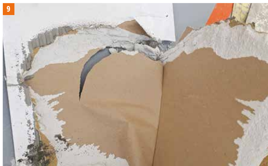
Photos 8, 9 Geoflex Express. Pull-off test on a tile after 1.5 hours, but with the maximum amount of mixing water (7.5 l/25 kg): the pull-off test caused the destruction of the substrate.
