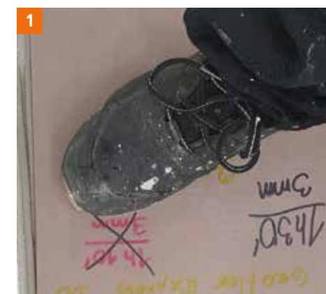
Photos 1, 2, 3 ATLAS Geoflex Express adhesive mortar - tiling in summer conditions, ambient temperature 28.5°C, layer thickness 3 mm, tests after 1.5 hours. From the left: 1. Load test (with rotation) - no sinking or loosening of the tile, 2. Pull-off test (with a handheld pull-off tester), 3. Hardness test - the trowel goes a few mm under the tile.
