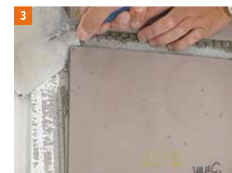
Photos 1, 2, 3 ATLAS Geoflex Express adhesive mortar - tiling in summer conditions, ambient temperature 28.5°C, layer thickness 3 mm, tests after 1.5 hours. From the left: 1. Load test (with rotation) - no sinking or loosening of the tile, 2. Pull-off test (with a handheld pull-off tester), 3. Hardness test - the trowel goes a few mm under the tile.
