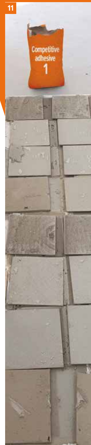
Photos 10, 11, 12 Pull-off test results for selected adhesives as shown in Fig. 1. Apart from the pull-off behaviour, attention should also be paid to the degree of adhesive discolouration under the tile, which indicates the rate of moisture loss in adhesive mortars, the increase in bond strength and the possibility of commencing grouting of ceramic coverings.
