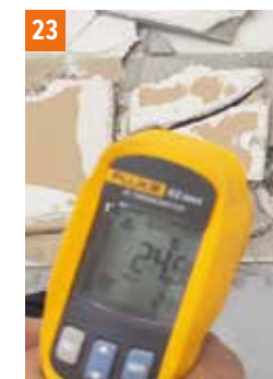
Photos 22, 23 Geoflex Express. The surface temperature of the tile within 5.5 hours of setting was stable and did not exceed 23.2°C for the 3 mm layer and 24.9°C for the 15 mm layer, i.e. a maximum of 4.7°C above the ambient temperature (heat of hydration). This indicates a stable progression of the hydration reaction.
