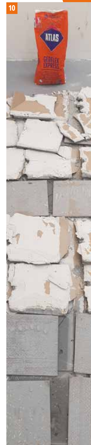
Photos 10, 11, 12 Pull-off test results for selected adhesives as shown in Fig. 1. Apart from the pull-off behaviour, attention should also be paid to the degree of adhesive discolouration under the tile, which indicates the rate of moisture loss in adhesive mortars, the increase in bond strength and the possibility of commencing grouting of ceramic coverings.
