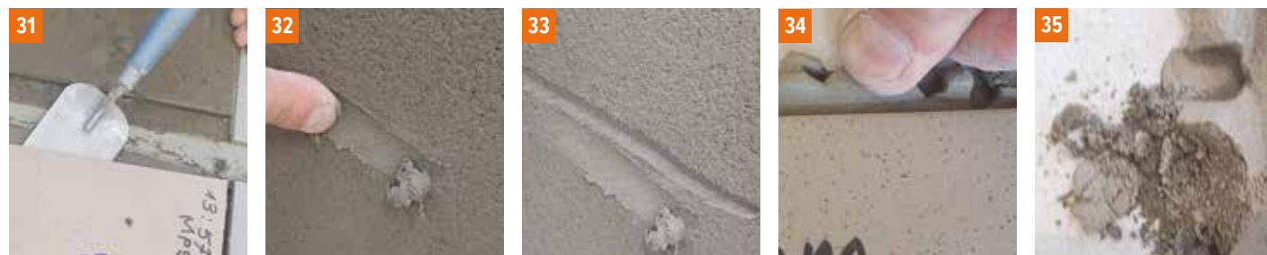
Photos 31, 32, 33 Fast-setting adhesive no. 1 (class "F") with a layer thickness of 15 mm - the setting process is comparable to that of traditional adhesives.
