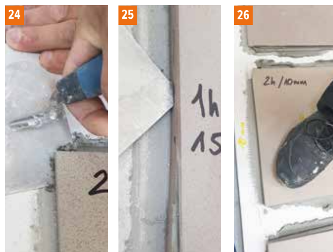
Photos 24, 25 Geoflex Express. With considerable force, it is possible to press the trowel into the adhesive mortar layer, regardless of its thickness of 3 or 15 mm. Photo 26 Regardless of the thickness of the mortar layer, abrupt treading on the tile and rotating the foot do not cause the tile to sink or move.
